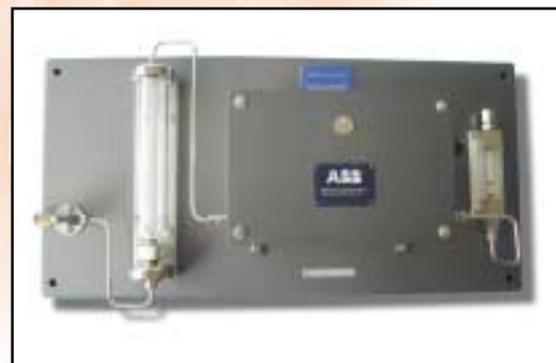
**System B** is ABB's traditional offering, and serves as the upgrade system for existing generators and new installations. This configuration employs one panel to measure 100%–85% or 85%–100% (fail-safe) hydrogen in air and is accompanied by a dual range analyzer panel for 0%–100% hydrogen in carbon dioxide and 0%–100% air in carbon dioxide.
